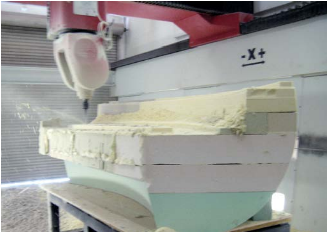
CNC-MILLING A PROTOTYPE FOR INSCAPE MEDITATION
