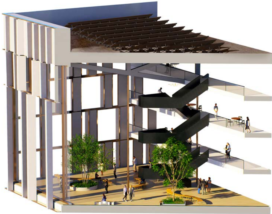
CANTILEVERED STEEL TRUSSES WITH FLOOR HANGERS
