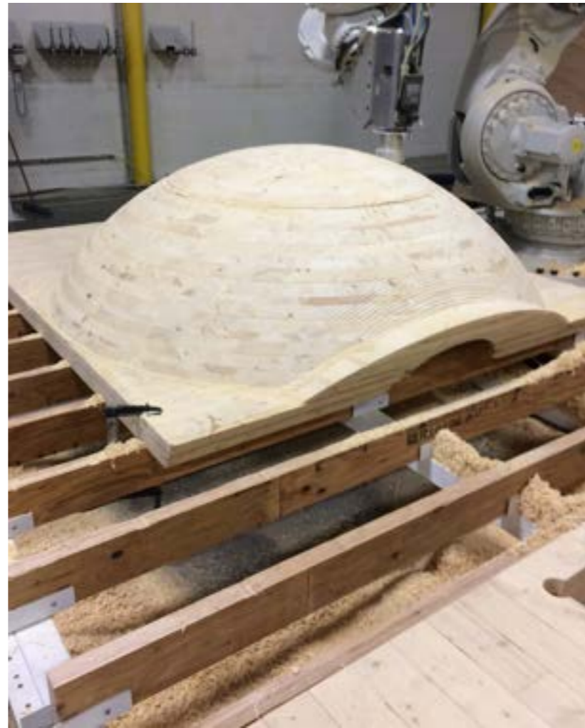
"Obolin," located at the Art Omi Sculpture and Architecture Park in upstate New York was fabricated from on sheet of CLT using a 7-axis robotic arm. The sculpture marks the exact locations of the sun during the Equinox and Summer and Winter Solstices. The materiality is the same as our proposed Wine Hotel.
