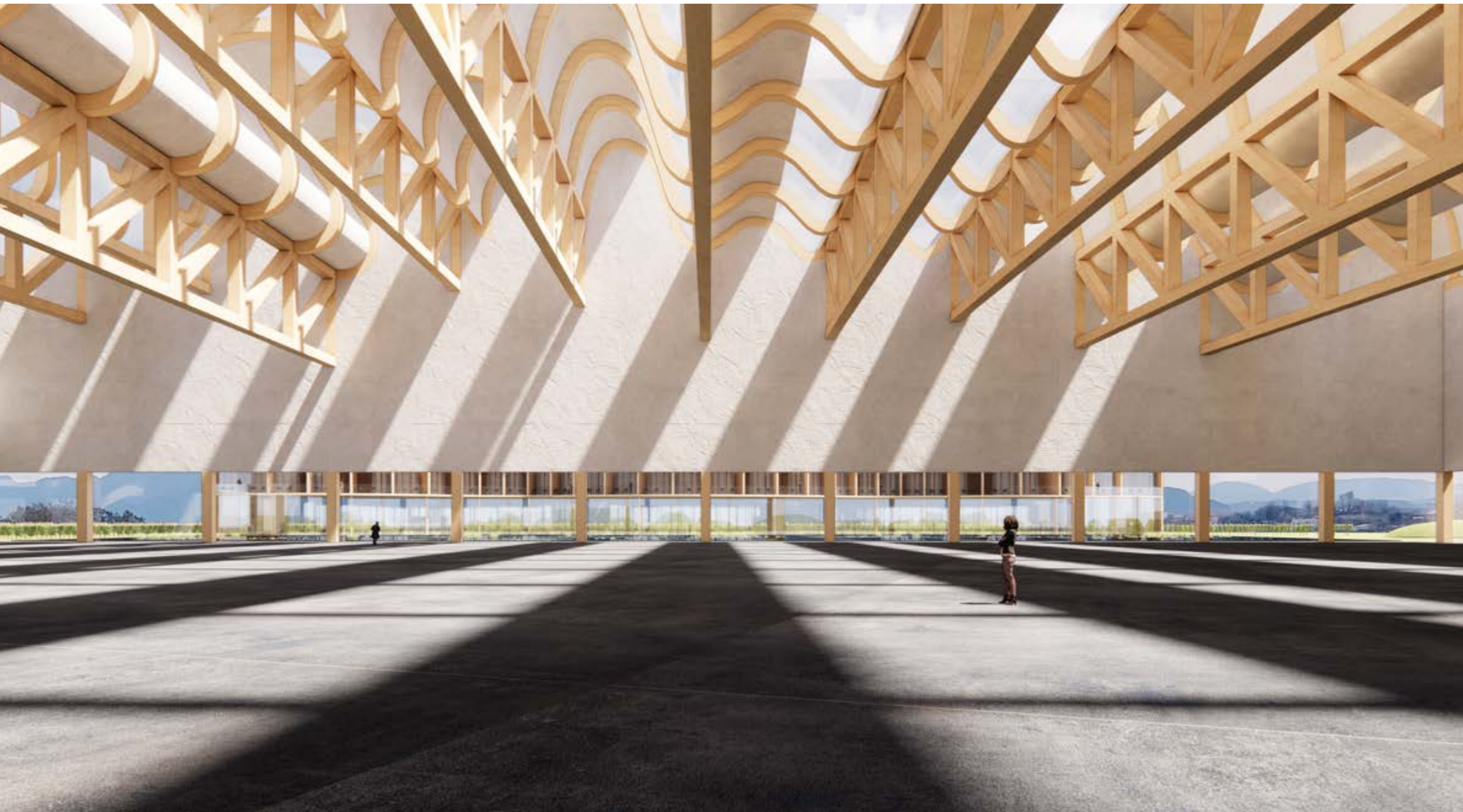
CLT truss modules are positioned at different heights according to the rhythm set by the "signature line," making it a truly unique space.
