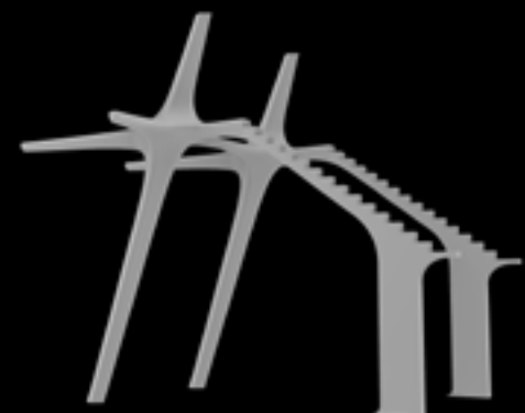
PRE-CAST CONCRETE STAND BEAMS
