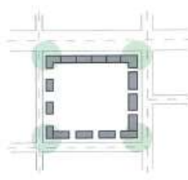
Step 5 This creates variety and flexibility within blocks. It's important that corners are always expressed with continuous building frontage as these are more visible and aid navigation within neighbourhoods. The boulevard must have 100% continuous frontage.
