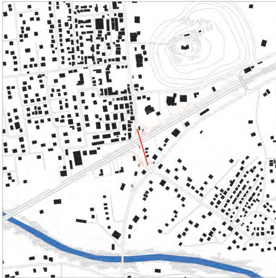
Erzen river, project plan 1. pedestrian/bike bridge 2. bus stop 3. pedestrian/bike loop 4. art stage
