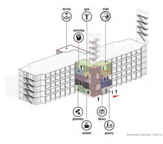
Round access\_Additions of a linear access balcony around the existing dormitory\_ Restoration of existing spaces (change in the typology of the room, addition of facilities such as kitchen 7 toilets)
